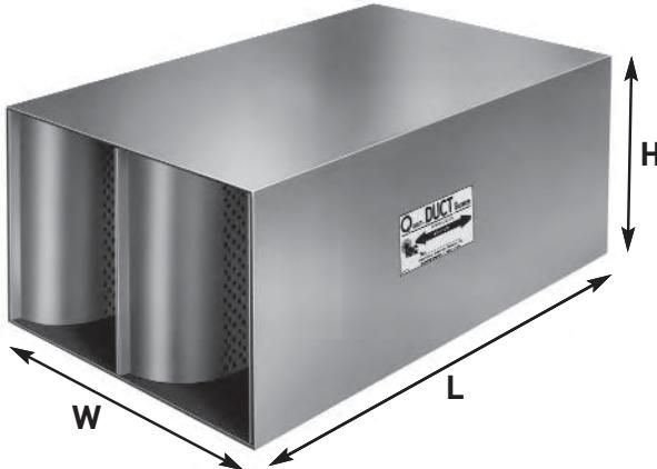
The IAC Type MS Quiet-Duct Silencers have been rated with procedures certified in accordance with applicable portions of ASTM E477. All Dynamic Insertion Loss and Self-Noise Acoustic Performance Data were obtained in a NVLAP accredited Aero-Acoustic Laboratory using the duct-to-room reverberant test facility **with air flowing through the silencers.**
