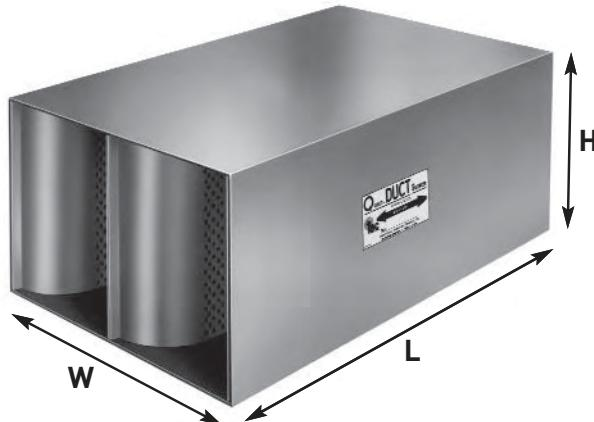
The IAC Type S Quiet-Duct Silencers have been rated with procedures certified in accordance with applicable portions of ASTM E477. All Dynamic Insertion Loss and Self-Noise Acoustic Performance Data were obtained in a NVLAP accredited Aero-Acoustic Laboratory using the duct-to-room reverberant test facility **with air flowing through the silencers.**
